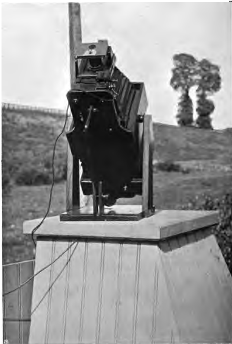
CAMERA FOR MEASURING ALTITUDES.
