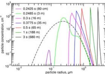
The figure shows results of microphysical calculations using a comprehensive gas-aerosol-ice trajectory model. Water condensation on liquid aerosol droplets, ice nucleation, and depositional growth of the ice crystals have been simulated, driven by one of the T- and p-trajectories close to the wing as shown above. The legend denotes distances behind the leading wing edge and times.
