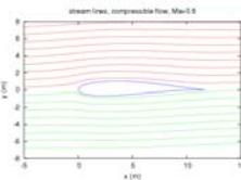
2-dimensional potential flow field (compressible flow) around a Joukowski airfoil, calculated with the method of singularities. Effective angle of attack: 1°. Mach number: 0.8. The dimensions of the airfoil are typical of a wide-body aircraft close to the fuselage.
